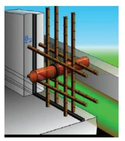
Joint surface must be clean and dry and any protrusions greater than 3 mm high ground or chipped off.
